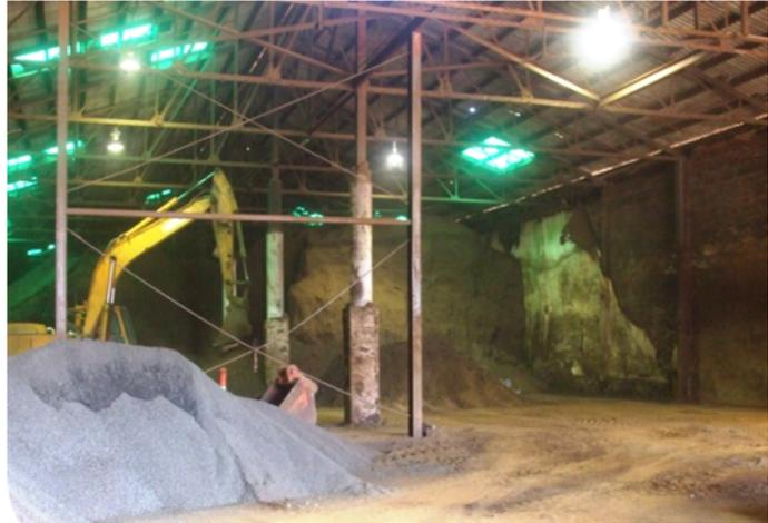
**Operations at the Victorian zinc oxide production site. Crushed Zeehan feedstock may be seen in the left foreground, with EAF dust stockpile excavation at rear.**
